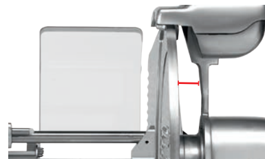
Increased gap between blade and machine body
