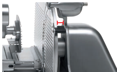
Increased gap between blade and machine body
