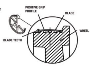
the balanced wheels provide a vibration free operation, and a positive grip profile on the border of the wheels assures a steady blade drive for a perfect cut, while protecting the blade teeth.
